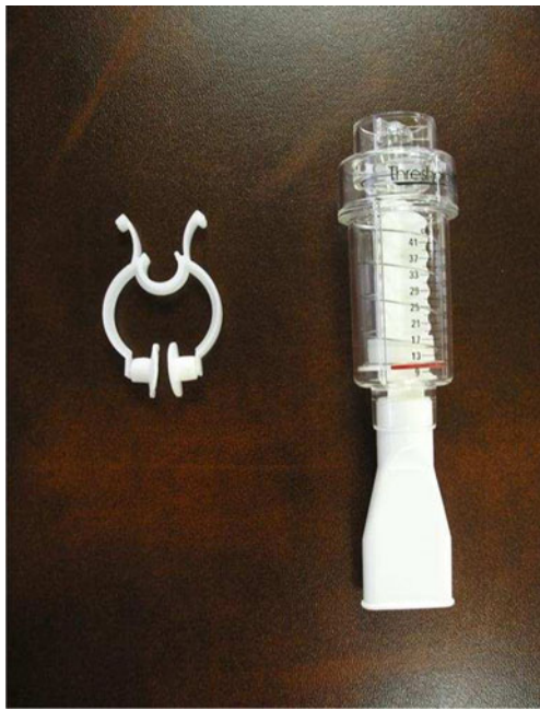
Fig. 1 Pulmonary trainer (Threshold IMT, Philips Respironics, Inc., Murrysville, PA, USA) provides consistent and specific pressure for inspiratory muscle strength and endurance training, regardless of how quickly or slowly patients breathe. This device incorporates a flow-independent one-way valve to ensure consistent resistance and features an adjustable specific pressure setting (in cm H 2 O) to be set by a healthcare professional. When patients inhale through Threshold IMT, a spring-loaded valve provides a resistance that exercises respiratory muscles through conditioning
