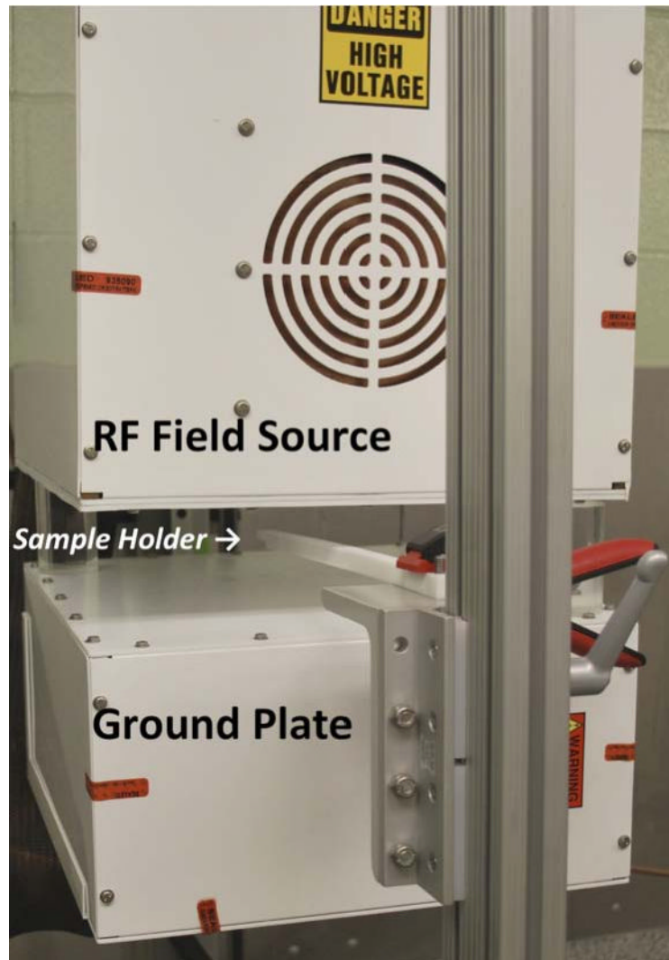
Figure 1. The 13.56 MHz RF field generator is seen with the Teflon sample holder in place. The air gap is approximately 10 cm between the transmitting and receiving heads.
