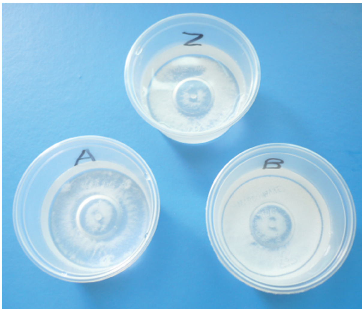
Fig. 2. Incomplete dissolution of stavudine capsules in water (Z = Zerit, A = Aspen Stavudine, B = Stavir).
