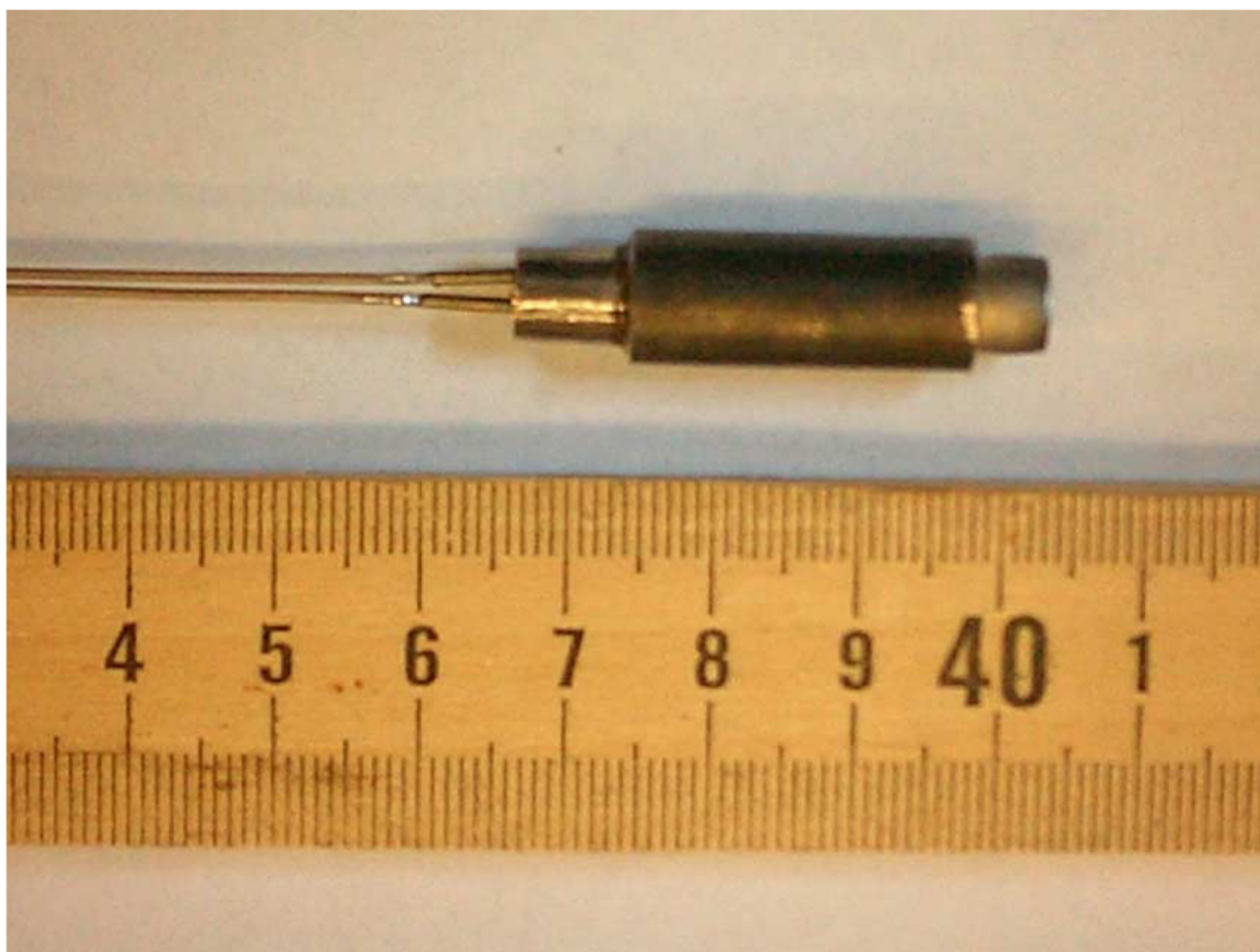
Fig. 3. Photograph of a splice assembly to join two multifilament MgB 2 wire inside Cu alloy matrix.
