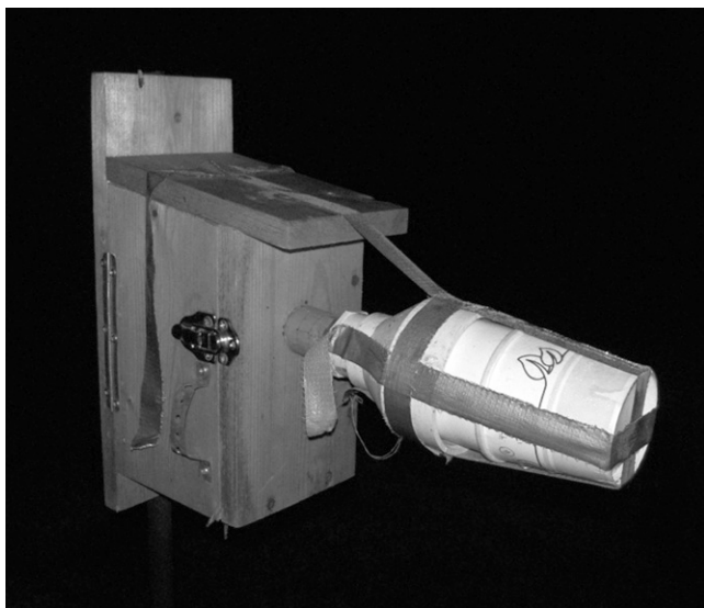
FIGURE 1. Eastern bluebird nest box with apparatus for introducing mosquitoes. The apparatus consisted of a plastic chamber (containing the mosquitoes), which fits into a plastic funnel inserted into the entrance hole of the best box.
