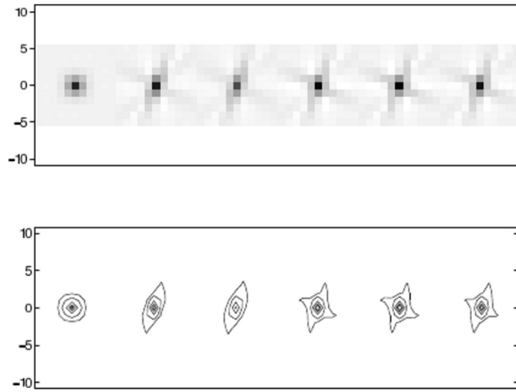
Fig. 13. Impulse Responses at (-130,100). From left to right, target, conventional regularization, certainty based regularization, AIMA regularization with \alpha = 0.1 , AIMA regularization with \alpha = 0 , FIN regularization with \alpha = 0 .
