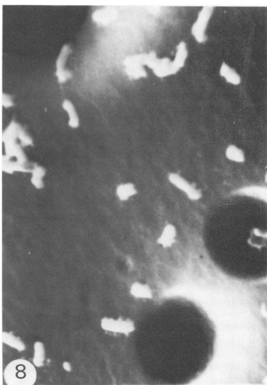
FIG. 5. Polycarbonate membrane (Nuclepore), 12.0- \mu\text{m} pore size, with 0.5- \mu\text{m} acrylic latex spheres. Latex particles thickly coat the cylindrical pores as well as the top surface. \times 5,000 .
