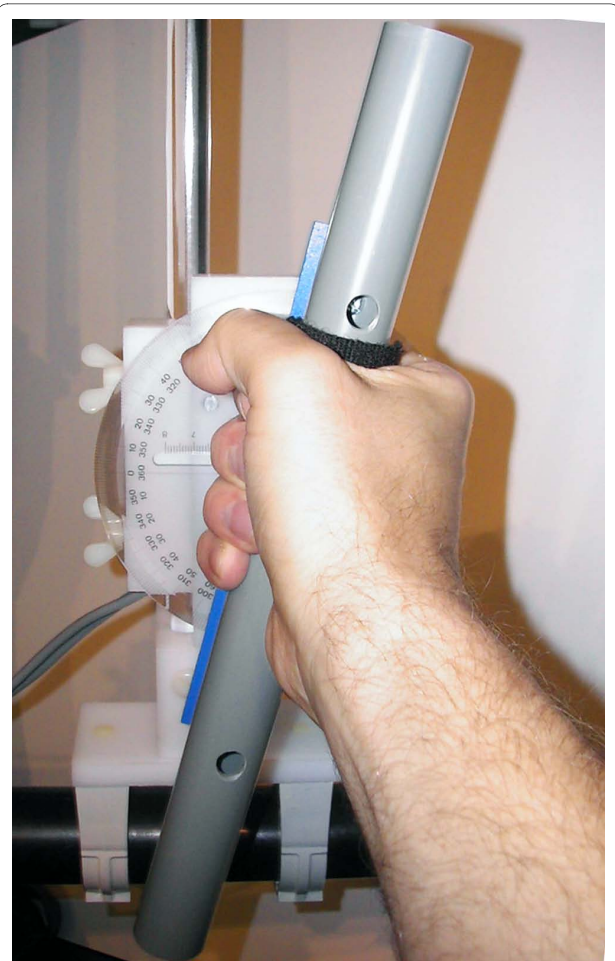
Figure 1 Illustration of the wrap grip, showing a subject folding the fingers and the thumb of the dominant right hand about the rod.
