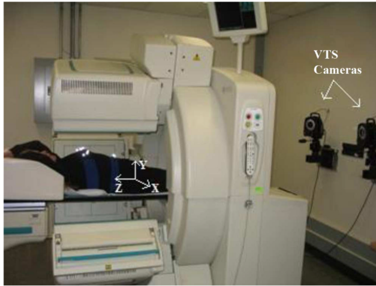
Fig. 1. SPECT and Vicon Visual Tracking System (VTS) setup. Two near-infrared cameras are mounted on the wall at the footend of the gantry. Three more cameras (not shown) are mounted on the wall at the head end of the gantry. The retroreflective markers on the belts may be seen as bright spots on the chest and the abdomen of the subject. The coordinate system for the VTS as calibrated to the SPECT coordinate system is shown with X being lateral, Y vertical, and Z axial. The arrows indicate the positive direction of the axes.
