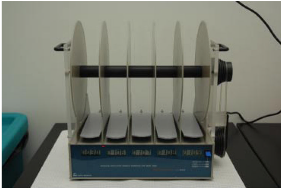
FIG. 3. Rotarod. The Ugo Basile/Stoelting rotarod is a rotating cylinder covered with grooved plastic divided into sections to allow testing multiple mice at one time. Mice walk forward on the cylinder as it rotates at a constant speed or at speeds increasing from 4 to 40 rpm over a 5-min test session. [Color figure can be viewed in the online issue, which is available at www.interscience.wiley.com .]
