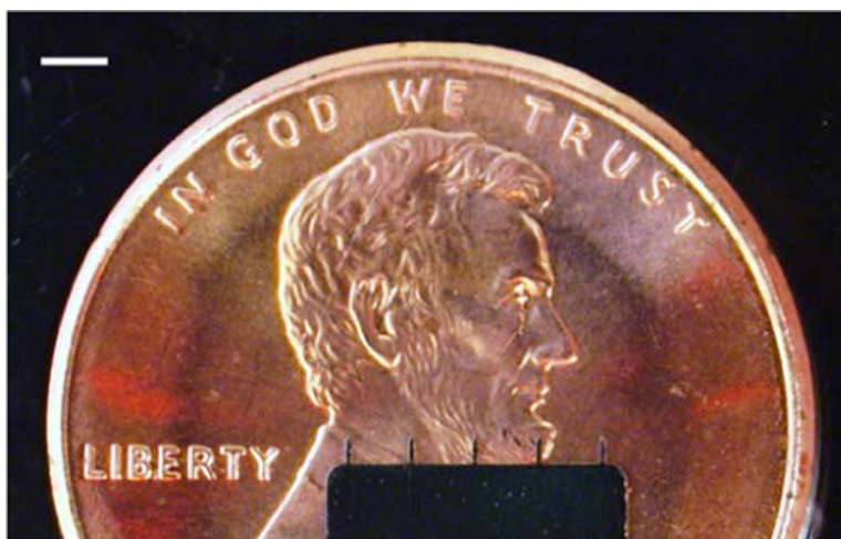
Fig. 1. Image of a microneedle array shown with a United States penny (scale bar = 2 mm).
