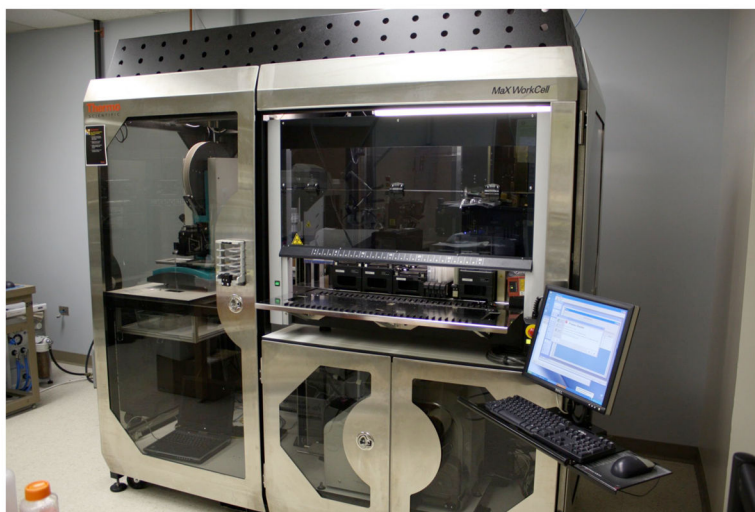
Figure 18. Automation of Crystallization Experiments. Crystallization robot in the laboratory of the author, the MaX WorkCell by Thermo Fisher Scientific Inc. The WorkCell integrates nanodrop setting (“Mosquito”, Molecular Dimensions Inc., Apopka, FL; on the left), liquid handling and screen preparation (“Starlet”, Hamilton Company, Reno, NV.; on the right), and sealing of crystallization plates (bottom right). The robot can handle a wide range of crystallization plates and formats and is typically combined with so-called storage hotels and a plate imager (not shown), that permit automated, periodic access to bar-coded plates and digital photography of individual droplets, respectively.
