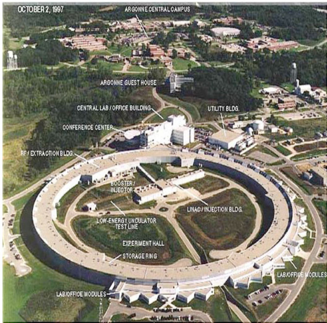
Figure 20. X-ray Synchrotron. Aerial view of the Advanced Photon Source (APS) at Argonne National Laboratory (Argonne, IL), a so-called 3rd generation X-ray synchrotron.
