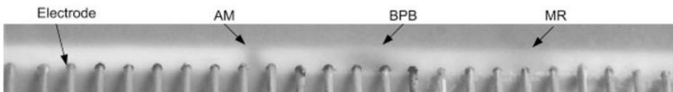
Figure 4. Separation of AM, BPB and MR in a membrane-less DFGF apparatus. The three dyes are well resolved and have band widths approximately equal to the distance between two electrodes (1.27 mm). The dyes were held within the separation channel under focusing conditions for greater than 10 h without noticeable signs of degradation or redox reactions on the electrodes. The electrodes within the separation channel are easily recognized.
