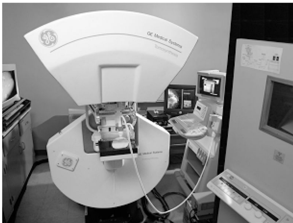
Figure 6. An early version of a combined tomosynthesis – ultrasound compression paddle system installed on a prototype tomosynthesis system developed at GE Global Research.
