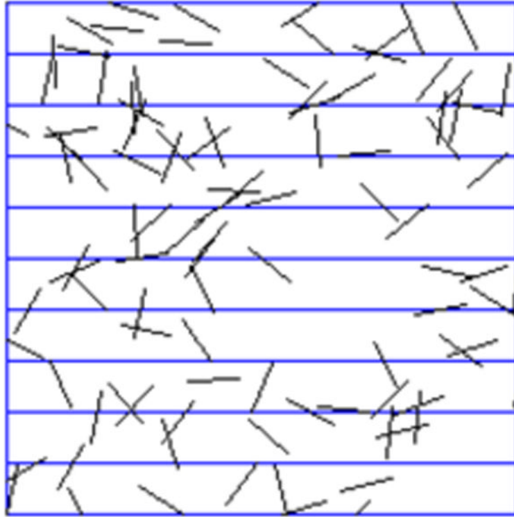
FIGURE 1. Buffon's Needle: after N tosses, the estimate for \pi is (2N/X) , where X is the number of times the needle intersects a line [2].
