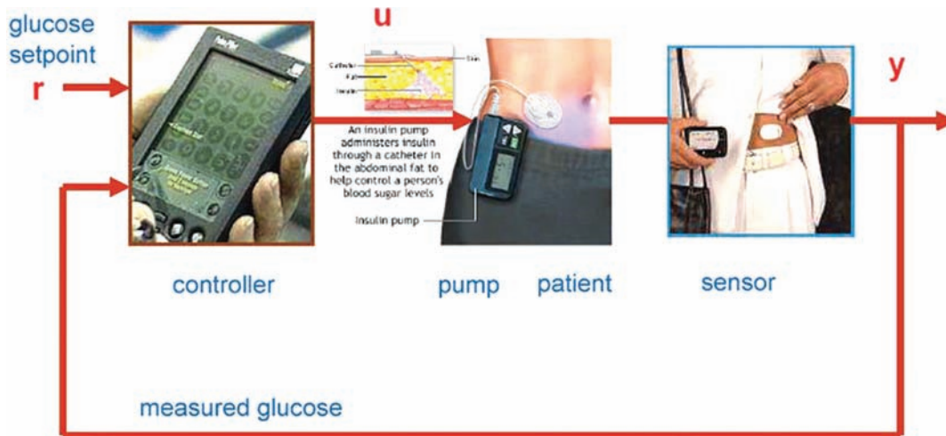
FIG. 1. The artificial pancreas, a closed-loop system for insulin delivery. The controller compares the desired glucose with the value obtained from a continuous glucose sensor. The controller output signal adjusts the rate of insulin delivered by an insulin infusion pump. The insulin affects the blood glucose, which is sensed and “fed-back” to the controller. Reprinted with permission from Bequette 1 and Mary Ann Liebert, Inc., New Rochelle, NY.
