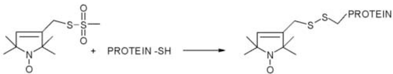
Figure 2. The methanethiosulfonate spin label and the side chain (R1) it generates.
