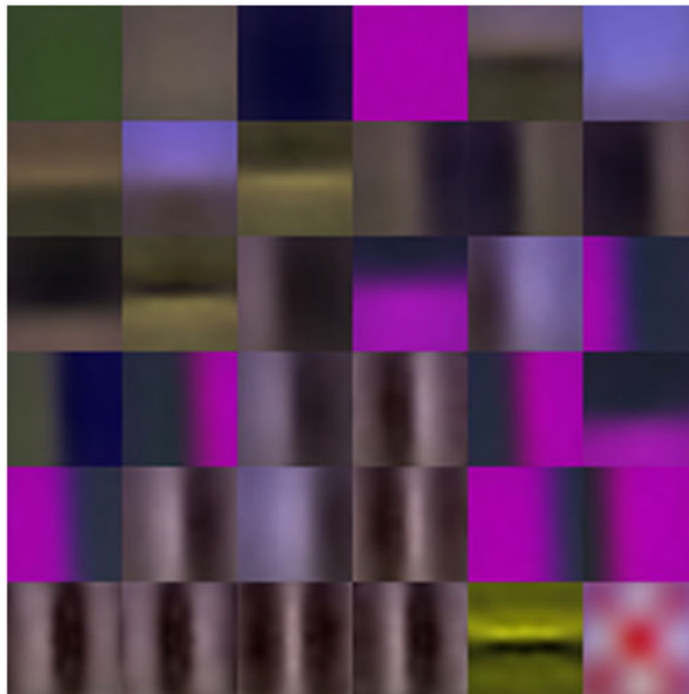
Fig. 8. The set of 36 cluster centers obtained from the image representation using the Gabor filters. These image patches are obtained by reprojecting the model simple cell responses at the center of the 36 clusters back into image space. These patches can be regarded as a set of features that can be utilized in representing the vast majority of image patches in the scenes of the visual world of the experiment. The patches are sorted in descending order of their relative frequency in all considered scenes from the top left corner to the bottom right corner.
