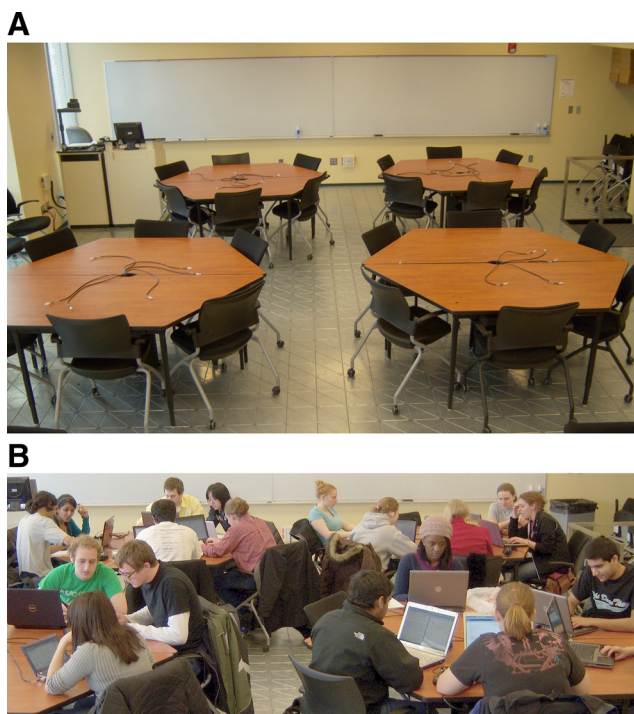
Figure 1. Classroom design to enhance teamwork and a continuous progress method of instruction. (A) Layout of the classroom. Each hexagonal table can be separated into two independent tables if necessary. Six Ethernet connections to the CWRU fiber optic network are shown. A power strip runs along the front side of each half table. (B) Students working in the classroom.
