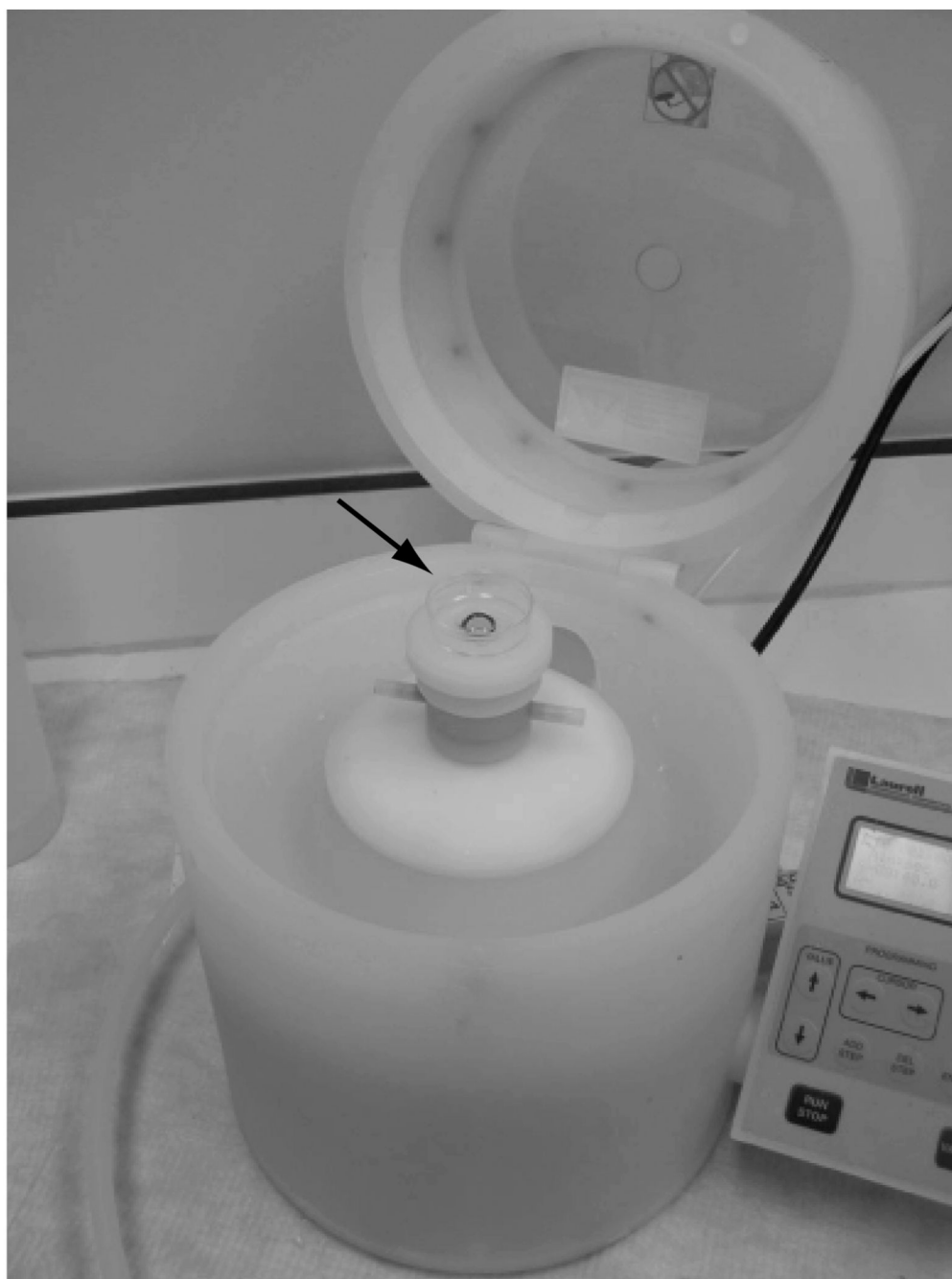
Figure 2. Laurel Technologies Spincoater with an “activated” MatTek dish in position before spincoating PVA/HCl solution. The chuck (arrow) can be changed according to the size required for the dish/disc being spun.
