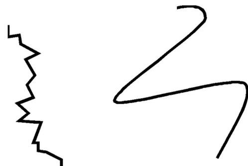
FIGURE 8. The difference between curvature tortuosity and length-ratio tortuosity. The branch segment on the left has higher curvature tortuosity and the branch segment on the right has a higher length-ratio tortuosity.
