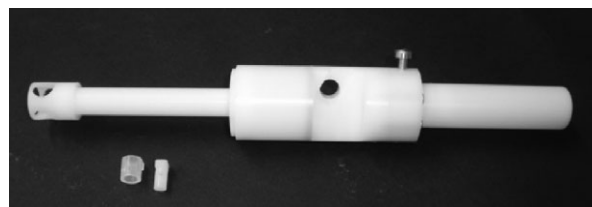
Figure 1. Photograph of the inline Venturi injection device with an 8 mm exit diameter used for the needle-free ballistic particle injection.
