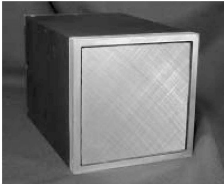
Fig. 1. Assembly drawing and photograph of FastSPECT II 3 × 3 modular gamma-ray camera.
