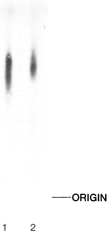
FIG. 4. TLC of the alkali-degraded lipid remaining after alkaline borohydride cleavage of the pure deacetylated polar PGL from serovar 9 (lane 1) and serovar 20 (lane 2). Plate was chromatographed in solvent B, sprayed with 0.1% orcinol in 40% \text{H}_2\text{SO}_4 , and heated.
