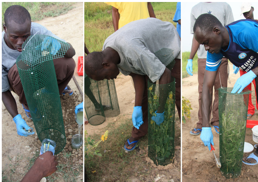
Figure 1 Picture of the type of glue trap used for testing mosquito attraction to local fruits/seedpods and flowering plants in Mali. The three pictures show how traps are mounted, how flowering plants are inserted, and how the outside of the trap is painted with glue.
