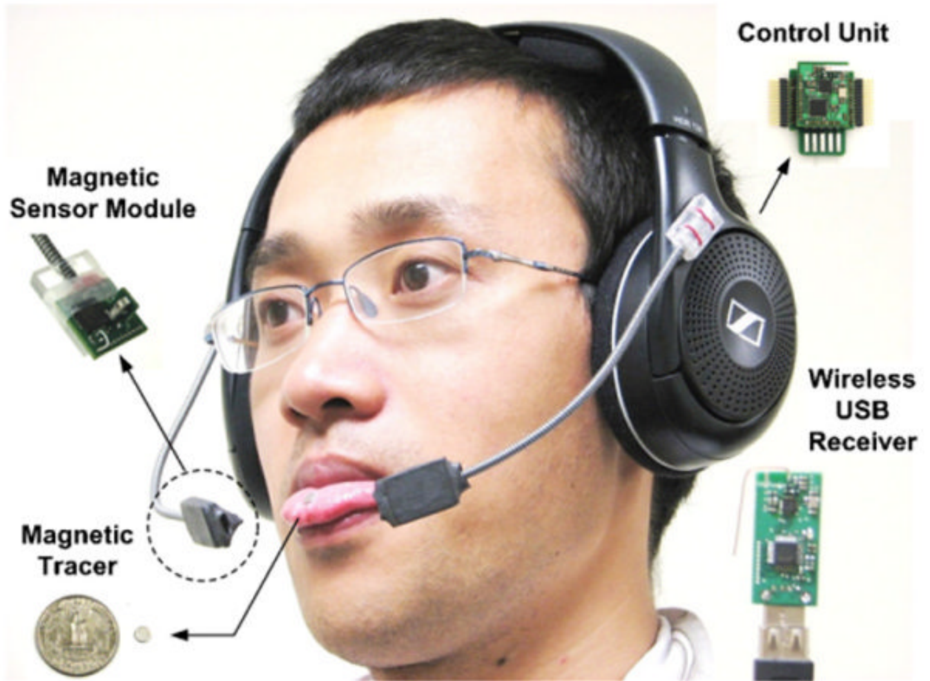
Figure 1. The latest external tongue drive system (eTDS) prototype and its main components, built using only commercial off-the-shelf components, including a wireless headphone.
