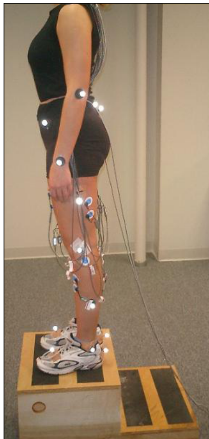
Figure 1. Participant with markers and electrodes preparing to perform a drop landing.
