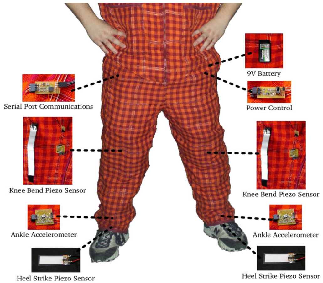
Fig. 1. Illustration of e-textile pants. (Only pants were used in the current study.)
