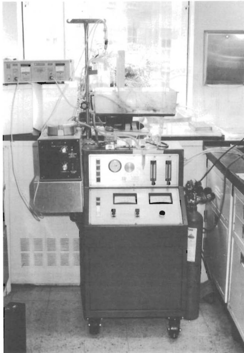
Figure 1. Photographic view of the liver perfusion and preservation system developed by modifying a kidney perfusion machine, model MOX-100 (Waters Instruments, Ltd, Rochester, MN).
