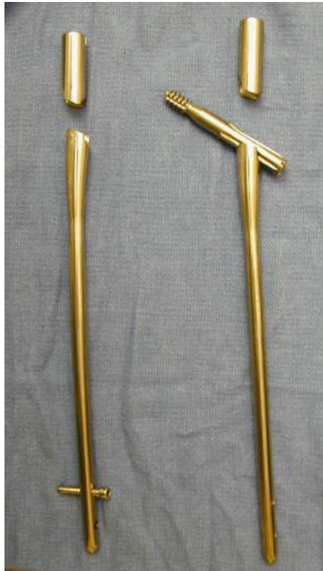
Figure 8. Two long gamma nails after removal demonstrating an identical obliquity and location of mechanical failure.
