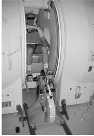
Figure 1. MR Compatible Exercise Cycle composed of plastic and wood was used to perform exercise for each participant in the 0.5T interventional magnet. Adjustments of resistance provided ability-appropriate exercise to reach target increase in heart rate of up to 50%.
