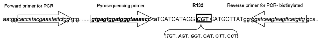
Figure 1. Schematic representation and primer localization. Map of the pyrosequencing assay for detection of codon transversion at positions 394 and 395 within exon 4, leading to the IDH1 R132 mutation. Primer-binding sites are depicted in lower case and the sequence to be analyzed in upper case . The mutation site assayed is highlighted by a box , below are the codons with the expected changes at the first and second positions, respectively. Arrows indicate the annealing positions of primer sequences from 5' to 3'.
