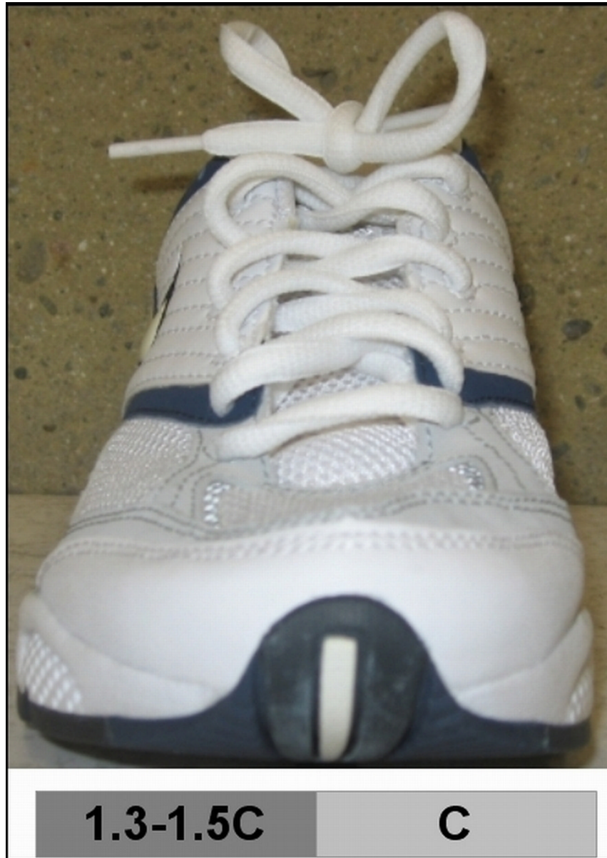
Figure 2. Variable-stiffness shoe with greater lateral sole stiffness (1.3-1.5 \times ) versus medial sole stiffness.
