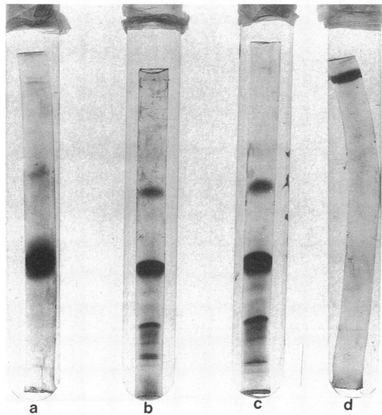
Figure 1. SDS-polyacrylamide electrophoresis. From left to right: (a) standard rabbit apolipoproteins A-I and E; (b and c) two different concentrations of the HDL-VHDL lipoprotein fraction used in our study; and (d) purified rabbit LDL. The figure shows total absence of apo B in our HDL-VHDL preparation.
