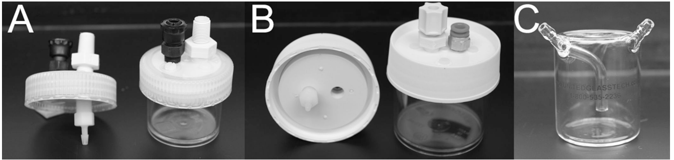
Figure 3. (A) Modified small polycarbonate reservoir, (B) Modified large polycarbonate reservoir, (C) Custom-made glass reservoir exclusively for liquid odorants.
