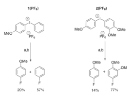
Figure 2. Observed regioselectivity for 1 (PF 6 ) (featuring the relatively electron-poor phenyl substituent) is worse than that of 2 (PF 6 ) (featuring relatively electron-rich 3,4-dimethoxyphenyl group.) a. TMAF/CH 3 CN, evaporation of solvent, addition of d 6 -benzene, filtration; b. 140 °C, 15 minutes.
