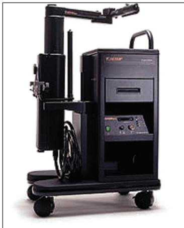
Figure 3: The AESOP system, Automated Endoscopic System for Optimal Positioning (Computer Motion, Goleta, CA)
