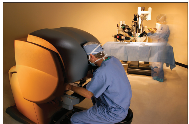
Figure 6: The original da Vinci robotic system (With permission from Intuitive Surgical Inc., Sunnyvale, CA)
