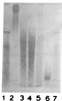
FIG. 1. Electrophoretic analysis of poly(A) before and after sonication. Polymer samples [200 \mu g in 20 \mu l of Tris-phosphate-EDTA gel buffer (19) with tracking dye] were applied to 8% polyacrylamide denaturing gels containing 8 M urea. Electrophoresis was done at 22°C, 150 V, and 35 mA for 5 hr. Gels were stained with 0.2% methylene blue. (Lanes 1 and 7) Yeast tRNA 3 eu , tRNA 1 gly , and 5S RNA M_r markers; (lane 2) poly(A) (dp \approx 550); (lane 3) poly(A) sonicated 7 hr; (lane 4) poly(A) sonicated 9 hr; (lane 5) poly(A) (dp \approx 120); and (lane 6) oligo(A) (dp = 17–29).
