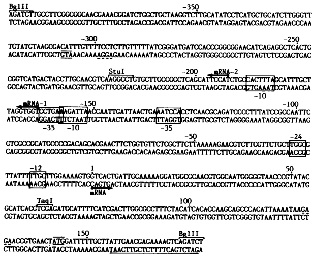
FIG. 2. Nucleotide sequence of the region containing the xylS and xylR promoters (11–13). Nucleotides are numbered from the transcription start site of xylS determined in this study, which is represented as 1. Arrows with a closed circle indicate the orientation and transcription start sites of xylR (mRNA-1, mRNA-2) (11) and xylS (mRNA). The underlined nucleotides are complementary to the 3' end of the 16S rRNA of Pseudomonas aeruginosa (14). The initiation codons (ATG) are both overlined and underlined. Sequences that are homologous to the consensus sequence of E. coli promoters (–35 and –10 regions) and of ntr/nif promoters (–24 and –12 region) are boxed. Restriction sites are shown with brackets above the sequence. The primer sequence used for reverse transcriptase mapping is doubly underlined.
