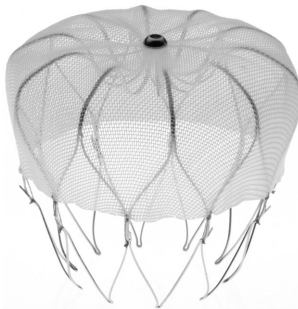
Figure 1. Watchman (Atritech) LAA closure device. A self-expanding nitinol frame structure with fixation bars and a permeable polyester fabric.
