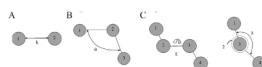
Fig. 17.1. Bonded interaction motions: (a) bond stretch is the movement between atoms directly bound to each other; (b) angle bend is a function of the relative position of atoms separated by one additional atom (1–3 pairs); (c) rotate-along-bond (dihedrals) is a function of the relative position of atoms separated by two additional atoms (1–4 pairs).
