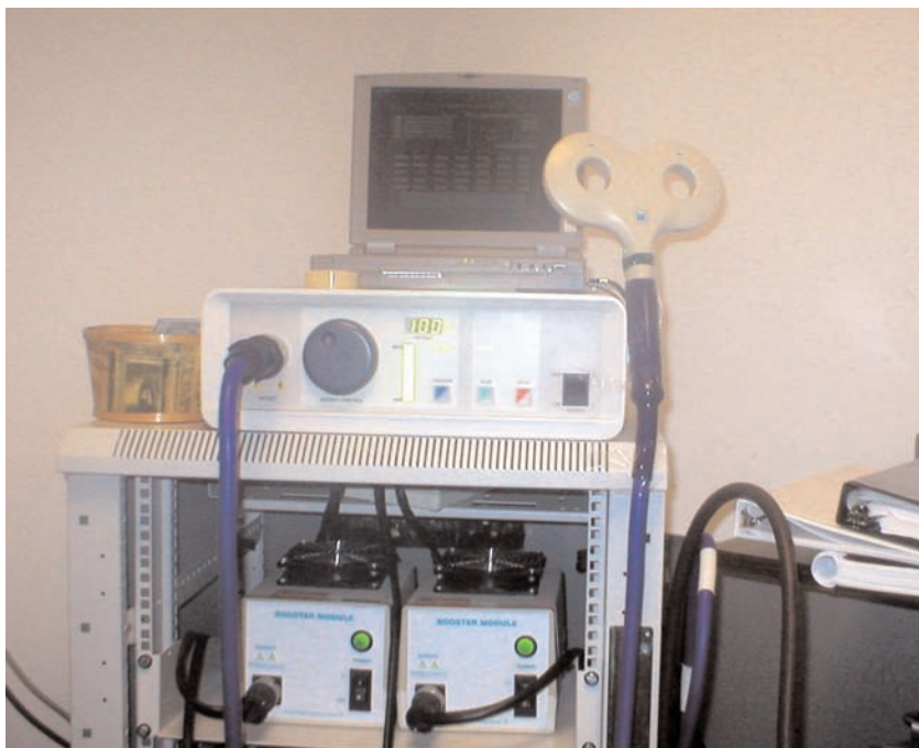
FIGURE 1. A MagStim TMS device with figure-eight shaped coil that is held flat against the scalp
