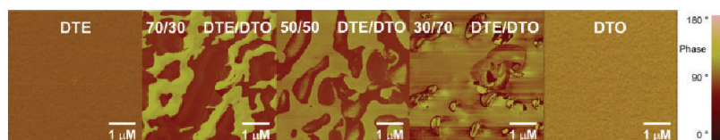
Figure 2. From left to right in the five 5 \times 5\text{-}\mu\text{m} AFM images shown above, the amount of DTO is increasing. The discrete DTE/DTO blends form phase-separated domains under in vacuo , 105^\circ\text{C} annealing conditions. The size and spacing of the domains are tunable by varying the composition of the blend. [Color figure can be viewed in the online issue, which is available at www.interscience.wiley.com .]
