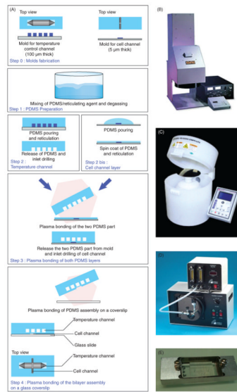
Fig. 2. The fabrication process. (A) Detailed fabrication procedure of the PDMS microfluidic temperature control device. (B) Photograph of the UV light source used to expose the patterns from the mask onto the wafer coated with photoresist (the future mold). (C) Photograph of the spin coater used to coat materials evenly onto surfaces. (D) Photograph of the plasma cleaner used to oxidize surfaces for subsequent bonding. (E) Photograph of a homemade coverslip holder.
