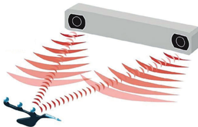
Figure 2 The optical tracking system requires a line of sight to the tracking beacons on the instruments it is tracking
