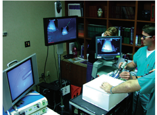
Figure 6 The physical layout of the experiment. The laparoscopic camera and ultrasound transducer are inserted through trocars into the white trainer box. The camera's video is viewed on the monitor (left) and the ultrasound video is viewed on the monitor (right). The central monitor provides the guidance software, in '3-D' as viewed through the stereoscopic glasses seen on the participant on the right
