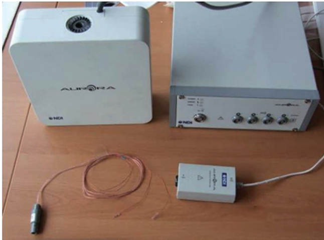
Figure 3 Book-sized magnetic field generator (left). This generator was placed next to the box trainer. The sensors were connected to the registration unit (right) that interfaced with the guidance computer
