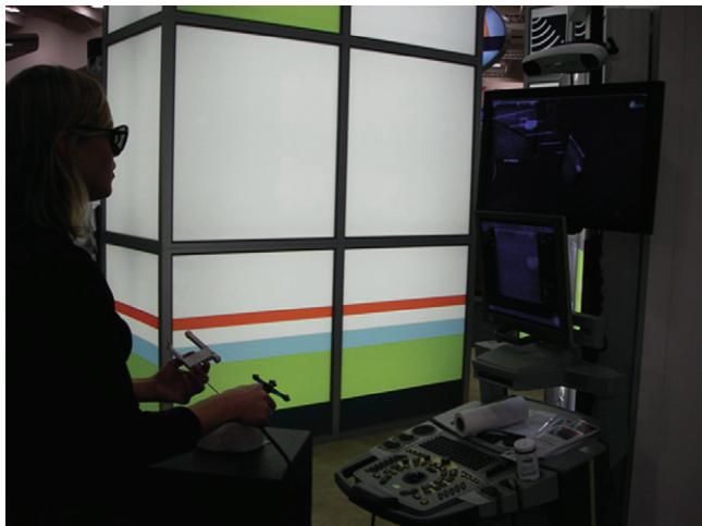
Figure 1 The guidance system based on optical infrared tracking. The user is holding a needle and ultrasound transducer, onto which are clipped tracking beacons. The motion of these beacons is observed by the infrared cameras (located within the white bar at top right), and their positions are triangulated. The guidance software represents the instruments in their actual spatial relationship, in real time, on the '3-D' monitor, which is viewed by the user through stereoscopic glasses
