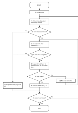
FIG. 1. Procedure to determining the imaging parameters k_y and z according to the current volume number v .
