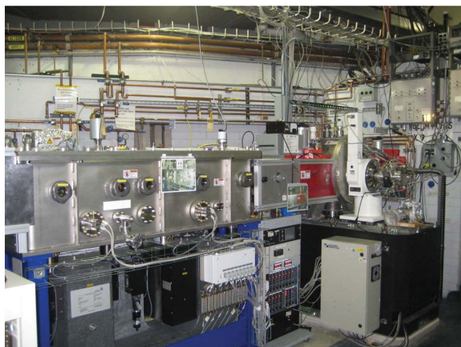
Figure 2 Photograph of the beamline optical components with the double-crystal monochromator (on the right) and the KB horizontal/vertical bimorph adaptive focusing mirrors (on the left).
