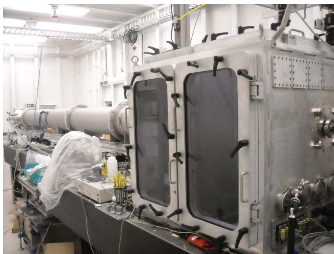
Figure 3 The long vacuum-compatible chamber of NLSL beamline X9 that contains both the SAXS (at the far end) and WAXS detectors (designed by Scott Coburn).
