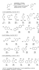
Fig. 3. Scope of the palladium-catalyzed trifluoromethylation of aryl and heteroaryl chlorides. Isolated yields are based upon an average of at least two runs. Minor amounts (2 to 5%) of reduced starting material (Ar-H) were usually observed. In a typical experiment, a solution of the palladium source and ligand 6 or 7 in dioxane was added to spray-dried KF and the aryl chloride. After addition of TESCf 3 , the reaction was stirred at 120 to 140 °C for 6 to 20 h. Because KF is hygroscopic, all reactions were set up in a nitrogen-filled glovebox in order to prevent the hydrolysis of TESCf 3 in the course of the reaction.
