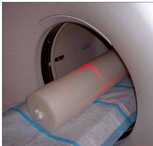
Figure 4: Experimental setup for scatter fraction (SF) and count rate (CR) performance test. Cylindrical polyethylene phantom (20 cm diameter and 70 cm length) with the line source inserted posteriorly was positioned at the center of scanner FOV
