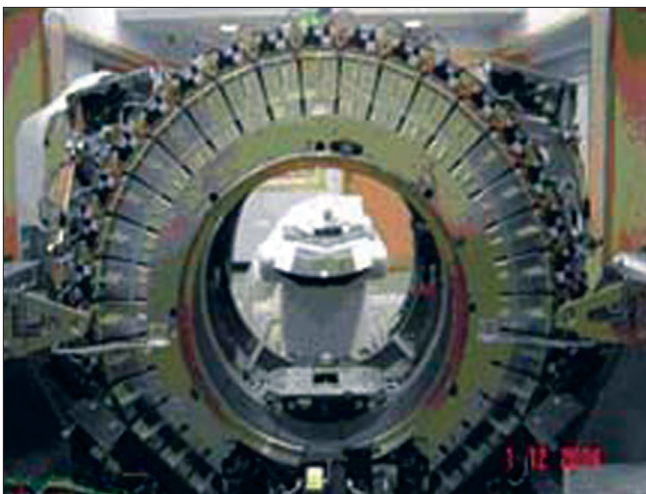
Figure 1: Arrangement of detector modules in D-ST PET rings
