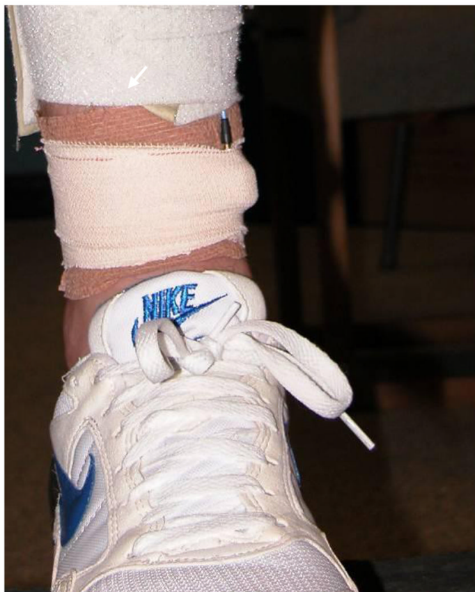
Fig. 1. Accelerometer taped to the anteromedial aspect of the subject's distal tibia.
