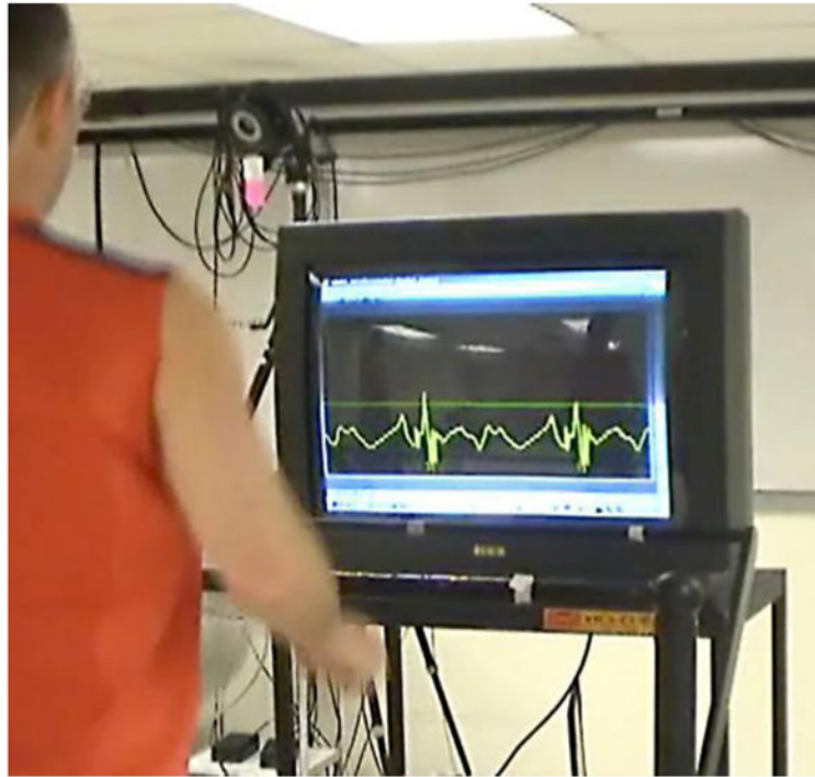
Fig. 3. Example of the real-time feedback from the accelerometer that was presented to subjects while they ran on the treadmill. Subjects were instructed to maintain their tibial acceleration below the horizontal line set at 50% of their peak values.
